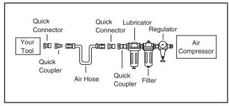
Figure 2. Installing your tool.
